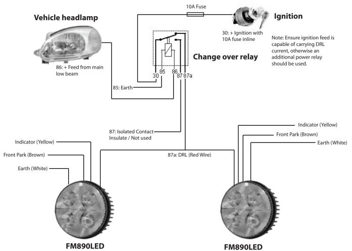
Note: Ensure DRL switches off when low / high beam of vehicle headlights are on. All other functions should operate as normal.
